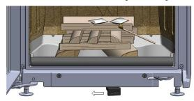
3. Let the first fire burn down with maximum air supply. This is to allow the stove to reach its operating temperature quickly. Light a new fire of the desired size. Wait a couple of minutes, until the fire has started burning properly. Then turn the damper to the left, until you have achieved a calm and harmonious fire.
