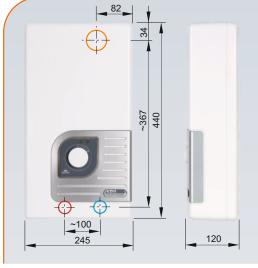
Supply water pressure 0,15 - 0,6 MPa Inlet and outlet section 1/2" \* inner thread
