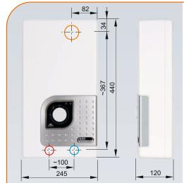
Supply water pressure 0,1 - 0,6 MPa Inlet and outlet section 1/2" \* inner thread
