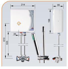
Supply water pressure 0,12 - 0,6 MPa Inlet and outlet section 1/2" outer thread Safety class IP 25
